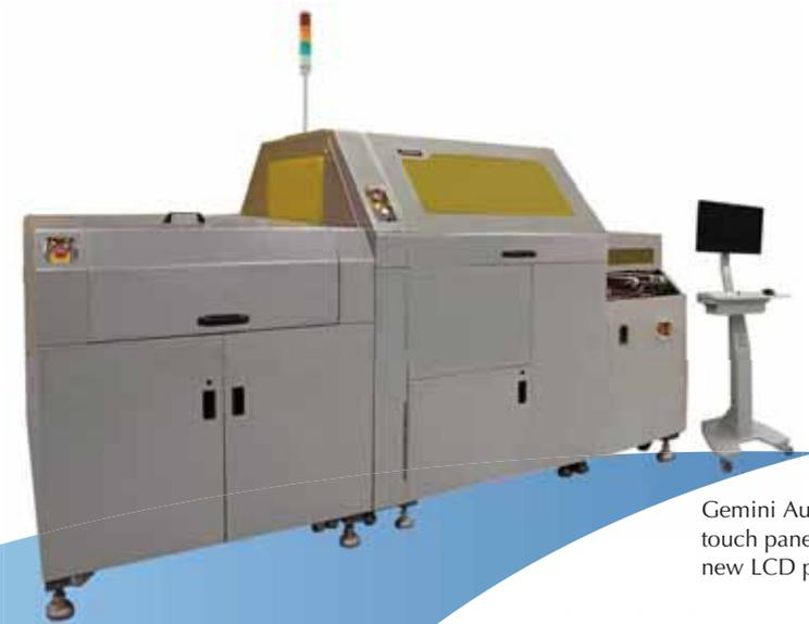
Gemini Automatic Panel Bonding System for touch panel, naked eye 3D display and other new LCD package lamination processes
