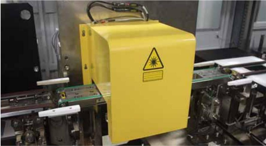
Solar WIS – resistivity and P/N type measurement
