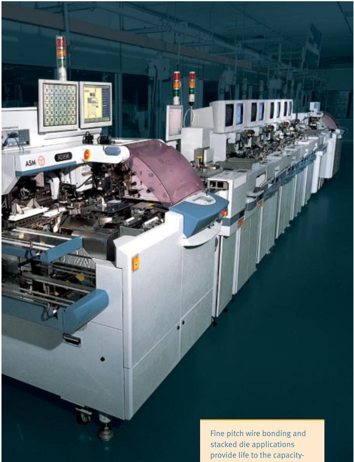
Fine pitch wire bonding and stacked die applications provide life to the capacity-driven wire and die bonder businesses.
